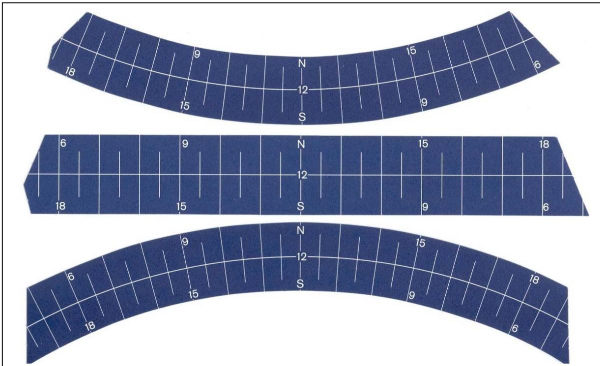
When putting in the charts, care should be taken that the 12-hour-line coincides exactly with the meridian line on the metal bowl (3). At a certain spot the metal bowl is provided with a hole (near the 14 o'clock line) through which the metal pin, which is suspended at the instrument by a chain, is to be inserted to such a depth that it pierces also through the paper chart which is thereby fastened.
