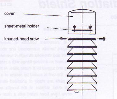
Remove the cover of the instrument by unscrewing the three knurled-head screws. Now the sheet-metal holder is exposed. Unscrew the two knurled-head screws and remove the sheet-metal holder.
